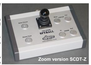
Model SCDT-Z has additional push button controls for operation of the zoom Spyball model SB-CZ functions as follows: automatic focus on / off, focus near, focus far, zoom in, zoom out and zoom fast / zoom slow.
