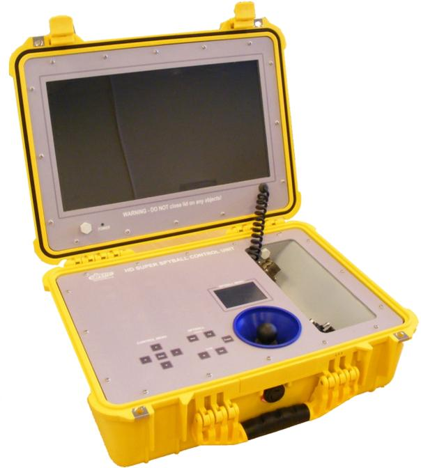
A 17.3 inch TFT colour LCD display mounted in the case lid behind a scratch resistant Polycarbonate window displays a clear and bright image from the Spyball camera even in bright sunlight.
