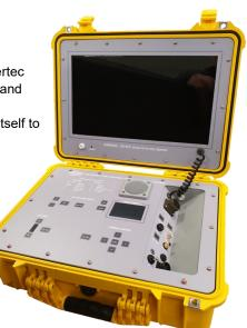
The built in Digital Video Recorder (DVR) stores 1080p MP4 video and 1920x1080 JPG photos to internal 256GB memory with simultaneous recording to removable USB Memory if required.
